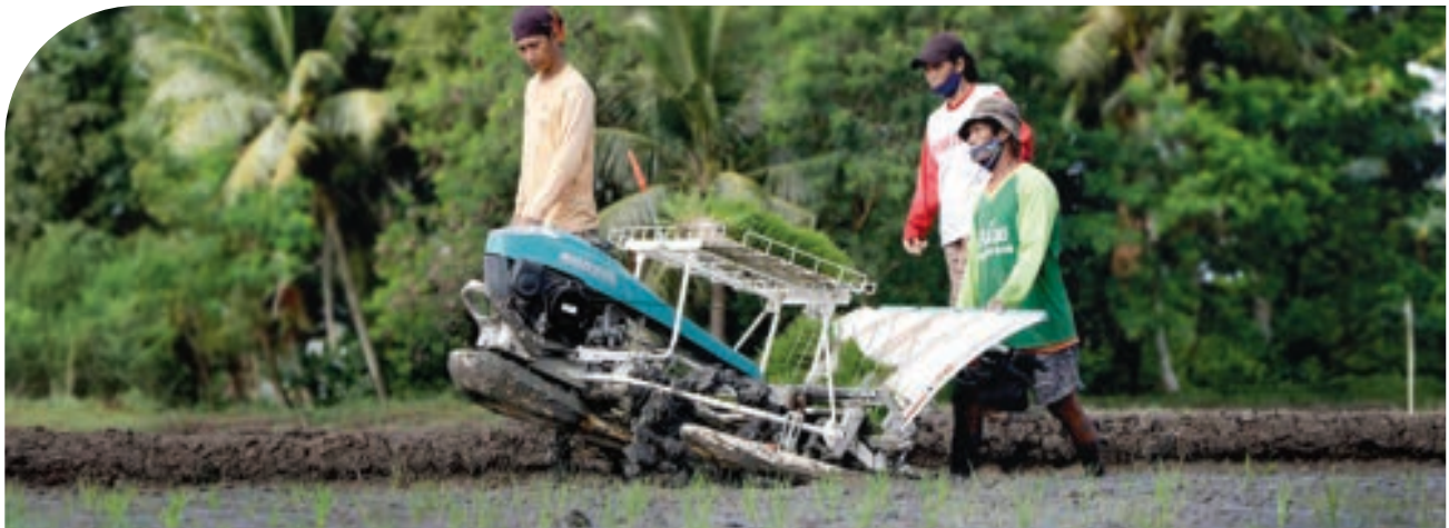
A farmer uses a mechanical transplanter for faster and more efficient rice seedling transplanting in Midsayap, Cotabato.
